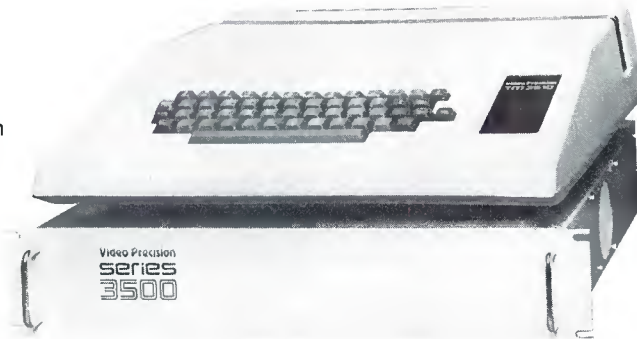
CG-3500 SERIES KEYBOARD AND ELECTRONICS UNIT
