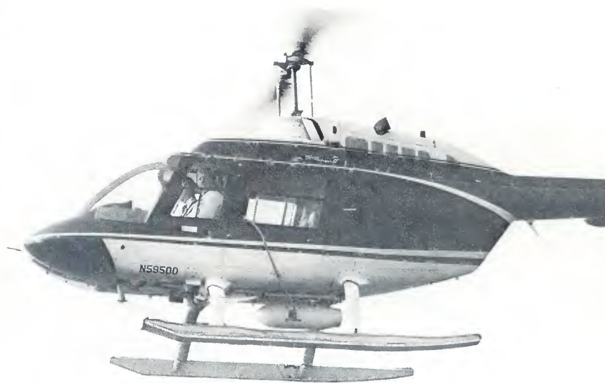
Mini Pod mounted on the cargo frame of a helicopter. Here there is no vulnerability to the type of damage that may be encountered with a more exposed antenna mounted on the landing gear.
