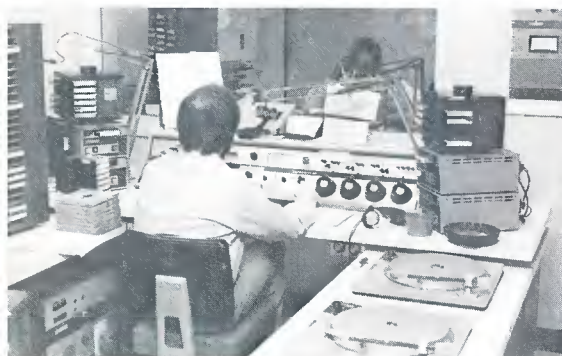
WLAP-AM control room with Jack Pattie, program director, at console viewing through window, Phil Miller, news director, during local newscast. Extended modulation meters and alarm panel in upper right. Lower left is remote control panel for equipment in other departments for use as needed.
